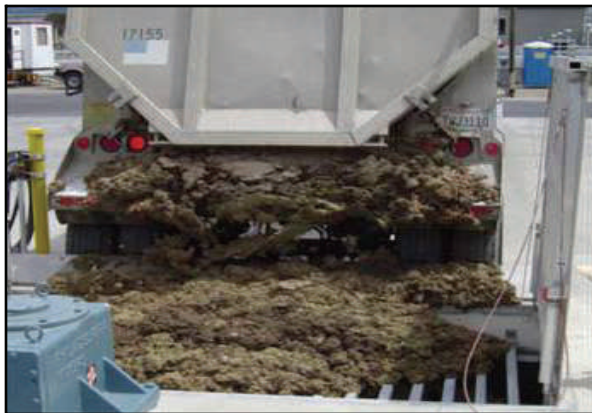
Food waste delivery to the East Bay Municipal Utility District's wastewater treatment plant. The food waste is collected by a hauler and pre-processed by screening, grinding, and removing metal pieces. A typical delivery is approximately 20 tons total weight
